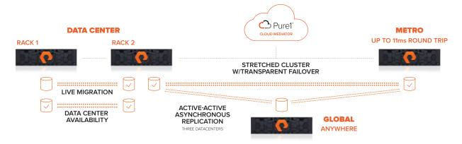
ActiveCluster has use cases within and between data centers. It enables live migration between any two FlashArrays, or rack-level HA clustering of four controllers for maximum resiliency. ActiveCluster really shines in the metro use case: simply take a running volume and "stretch" it between two sites separated by as much as 11ms of latency, with zero additional configuration required.
